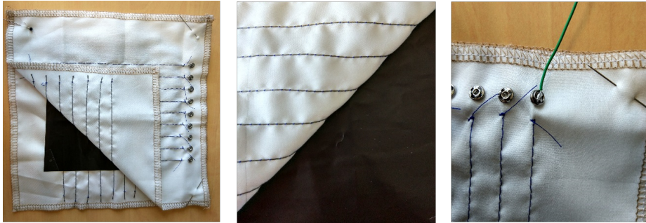
Fig. 3. From left to right: overview of the Velostat layer, close up of Velostat sheet and fabric underneath, close up of the detachable clips.
