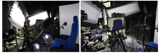
Figure 3: Our photogrammetry setup for scanning users' face composed of fourteen DSLRs and seven light sources covered with diffuser sheets.
