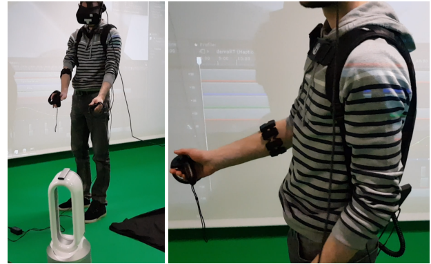
Figure 6: User equipped with haptic devices: vibrating controllers, vibrating armband, vibrating backpack. A fan providing wind and heat is also plugged in.
